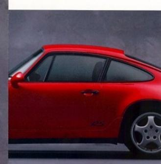
The fixed rear spoiler provides precisely the amount of downforce to counteract lift forces at speed. An experienced driver can feel the spoiler's effect at speeds as low as 45 to 50 mph.
